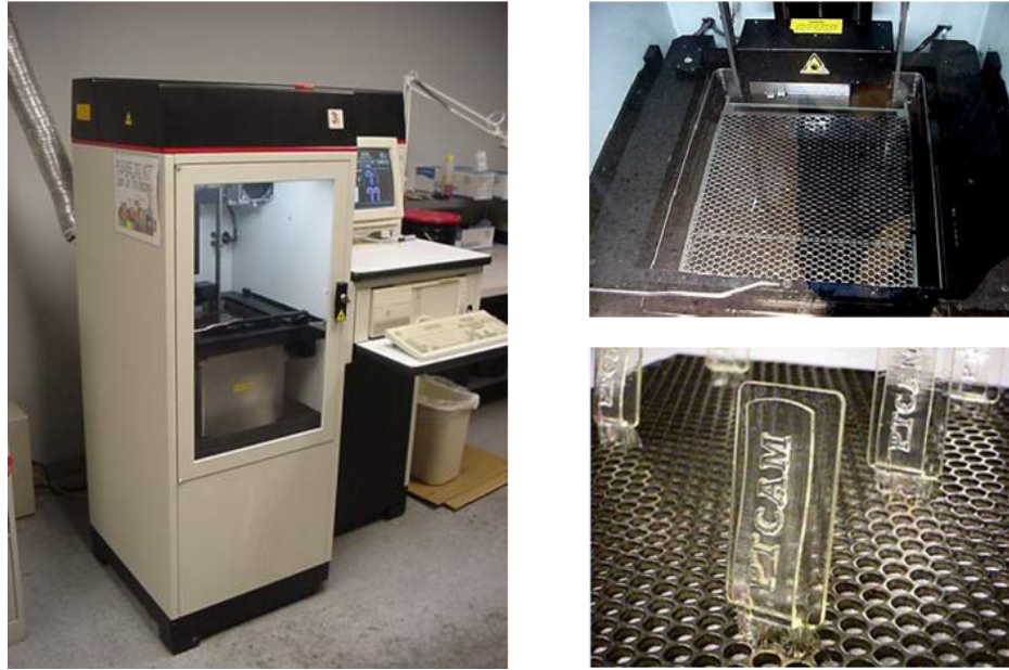
Figure 1.2: 3D Systems stereolithography machine (left), its photopolymer platform (right top), and the end of a print run process (right bottom). (Images courtesy of PT CAM, Inc.)
